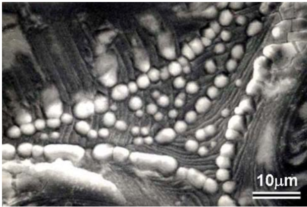
Fig. 10 Small \text{Cu}_2\text{O} balls solidified along the grain boundary of recrystallized copper without bonding. After tough-pitch copper was kept in the liquid \text{Cu} + \text{Cu}(\text{O}) area of the \text{Cu}-\text{O} phase diagram, liquid \text{Cu} changed to \text{Cu}_2\text{O} through a hypo-eutectic reaction. Molten \text{Cu} + \text{Cu}(\text{O}) changed to \text{Cu}_2\text{O} + \text{Cu}(\text{O}) below 1065^\circ\text{C} following the eutectic reaction
